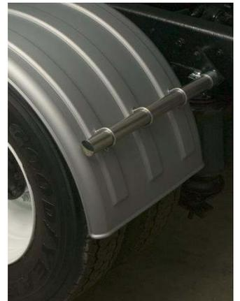
**NOTE:** Depending on the length of the truck frame and the placement of the mud flap hangers, the fender may tuck inside the mud flap hanger.
