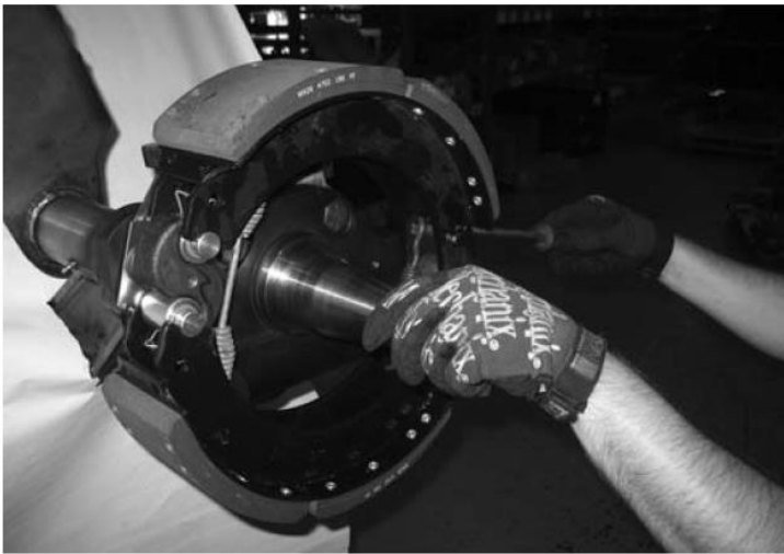
Figure 5 - Remove retainer springs
