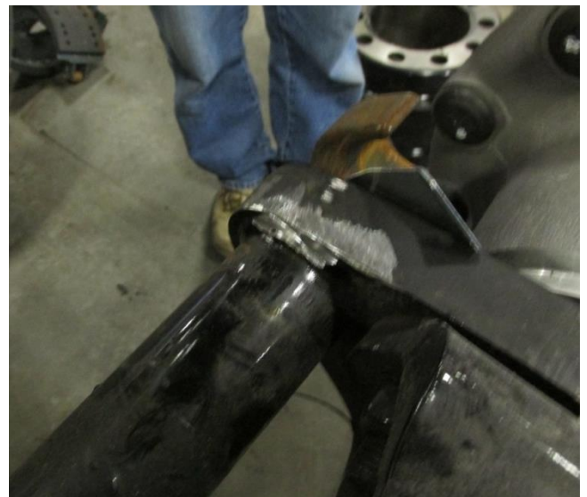
Figure 3 - Weld bead around brake cam tube
