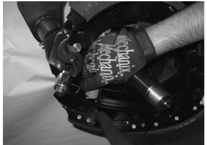
Figure 6 - Remove return spring and upper shoe
