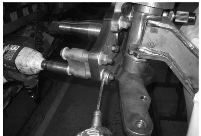
Figure 7 - Remove anchor bolts
