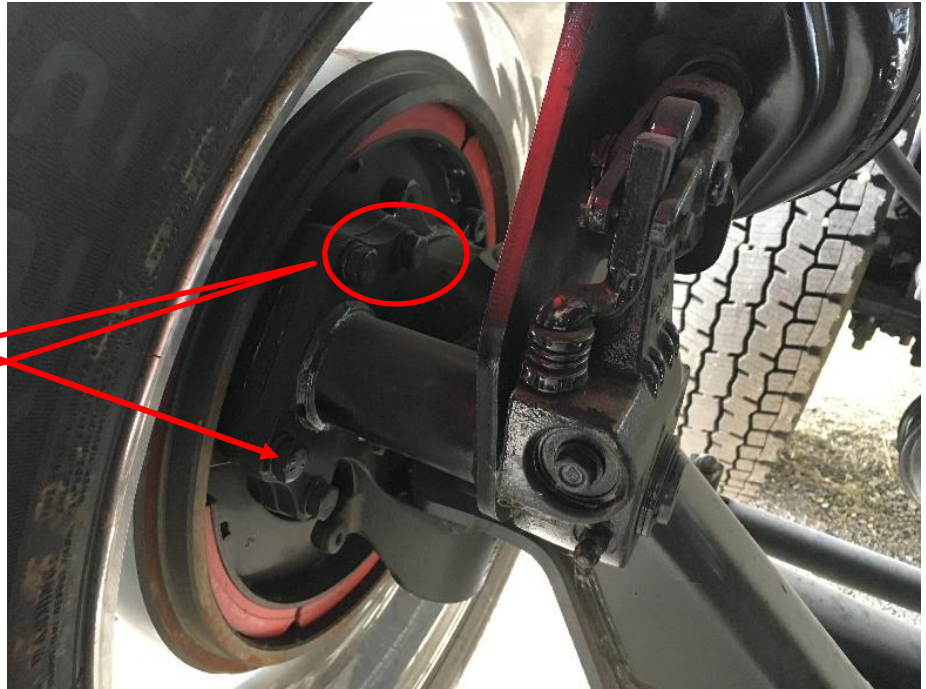
Figure 4 - Brake Cam Tube Mounting Bolts
