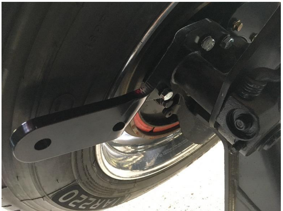
Figure 5 – View of Right Front Fender Bracket PB62R Installed
