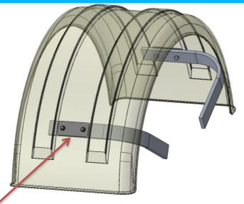
ALIGN STEEL PLATE WITH ALUM. ARM
