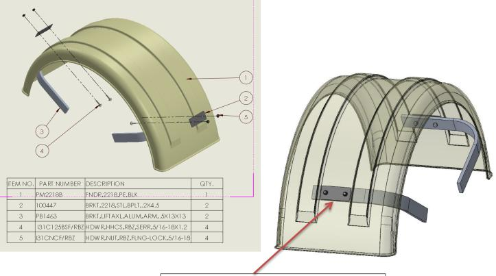
ALIGN STEEL PLATE WITH ALUM ARM
