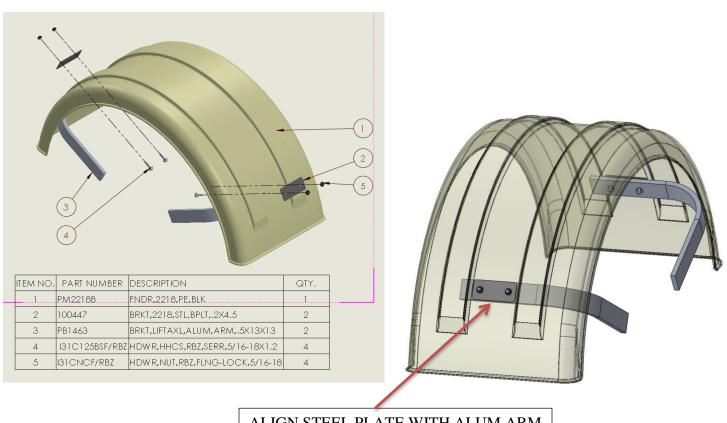
ALIGN STEEL PLATE WITH ALUM ARM
