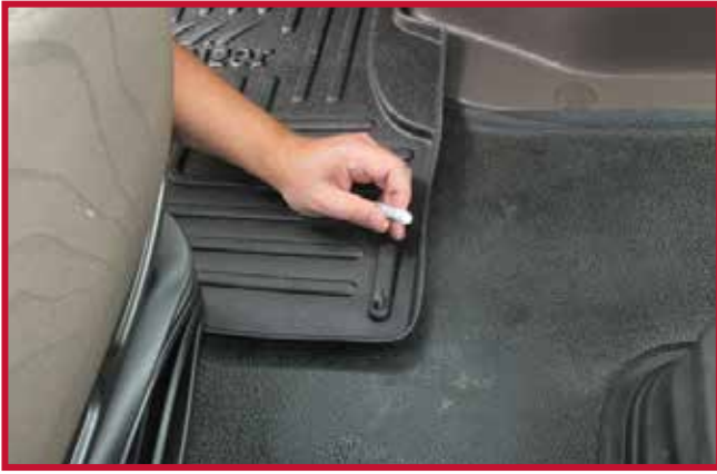
Figure 6 - Confirm Location Driver Mat and Hook
