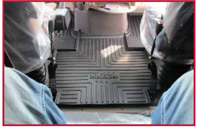
Figure 8 - Center Mat Installed
