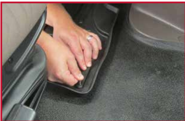
Figure 7 - Apply Pressure to Hook
