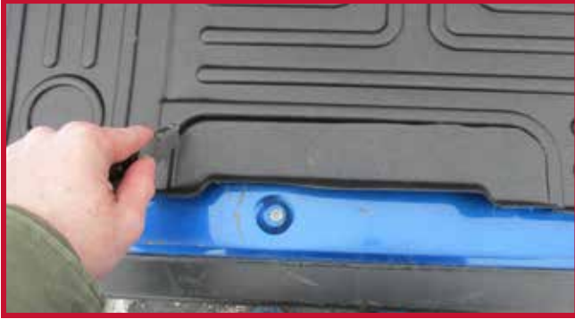
Figure 7 - Driver Mat Trimming Diagram
